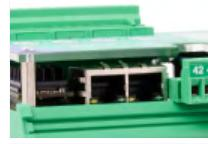
**2x EtherCAT ports + RS485 + Analog output**
