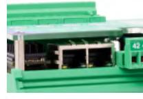
**2x POWERLINK ports + RS485 + Analog output**
