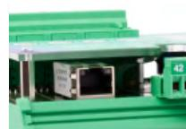
**Modbus/TCP port + RS485 + Analog output**
