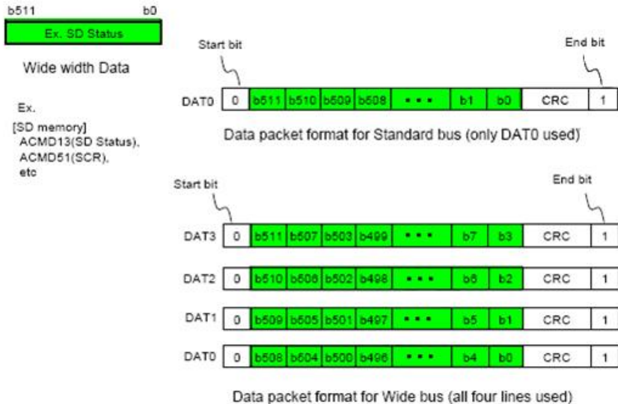
Figure 6-7: Data packet format - Wide width data
